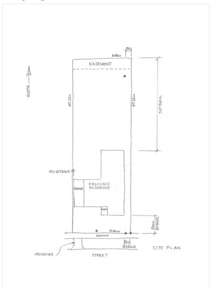
This is a sketch of a site plan at the concept stage showing the site details for the proposed building and a further explanation for each of these details. The site is a long narrow block which runs north—south. The proposed building is a single storey residence with an attached single garage. It is sited on the front half of the block, facing south.
