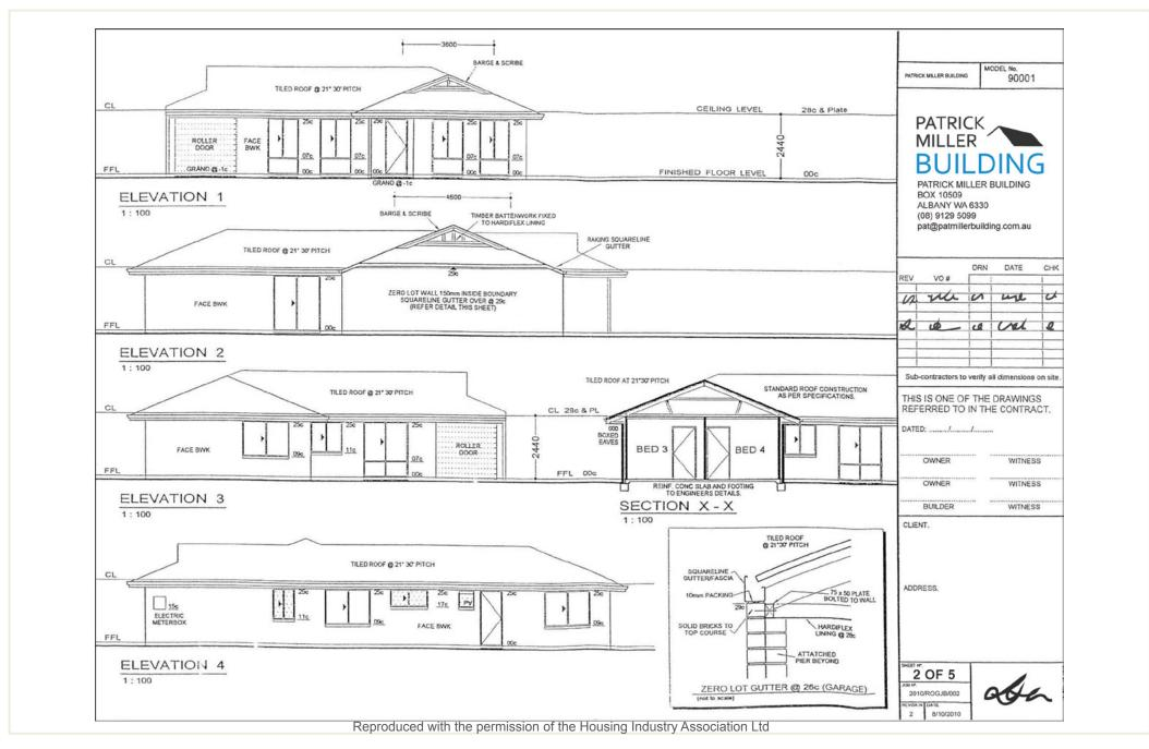
This is an elevations drawing from the design development stage showing all four elevations of the proposed residence. External details are shown including windows, doors and roof. Floor and ceiling heights are included. It also shows a section through, depicting the internal wall and doors for bedroom three and four. There is a detail drawing showing the guttering. The completed title block is on the right hand side of the sheet.
