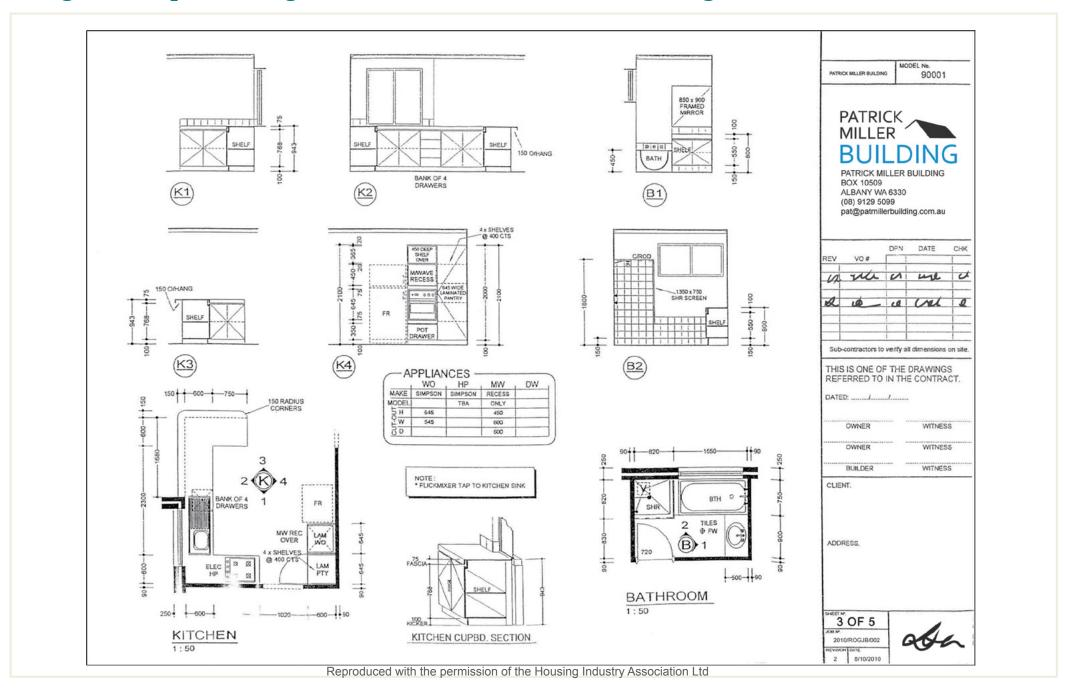
This is a working drawing of internal details and section-throughs from the design development stage. It shows detailed information for the internal fitout, including location, dimensions and types of cabinetry, appliances and fixtures.
